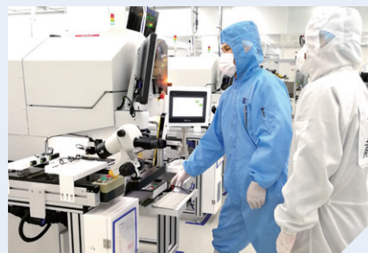
The production line of the packaging & testing of IGBT modules
